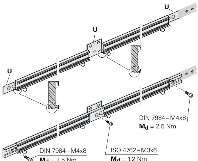
Starting from the center, evenly press the scale-tape carriers onto the mounting surface using the roller.
