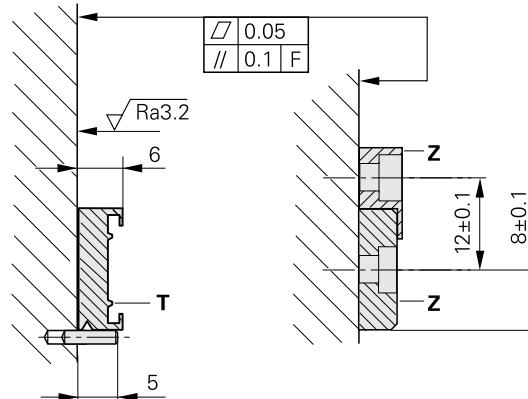
Attach the stop pins or the stop rail.
