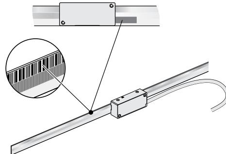
Insert the scale tape in the scale-tape carrier (do not bend it).
