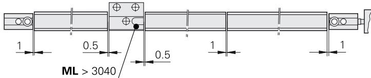
Make sure that the scale-tape carriers are positioned correctly.
