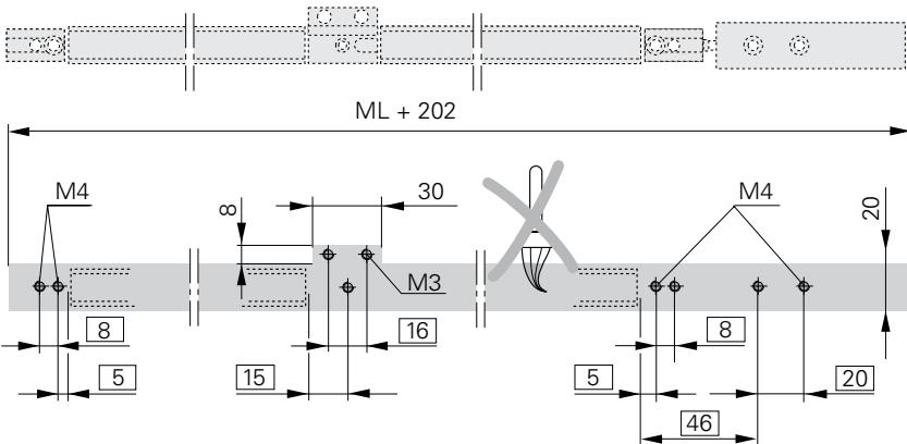
The scale tape carrier with PRECIMET adhesive mounting film has to be attached at a temperature  $> 15^{\circ}\text{C}$ ! Pay attention to the expiration date on the package! Peel off the protective film from the mounting film, protect the adhesive surface from contamination!
